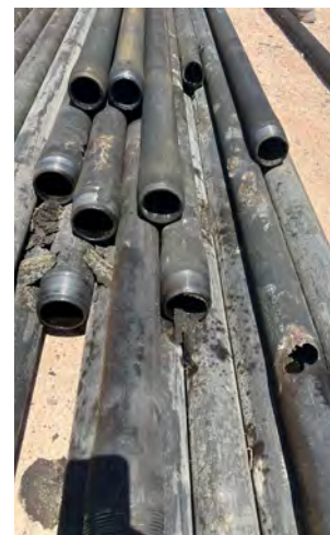
Figure 8. Corroded Production Tubing
