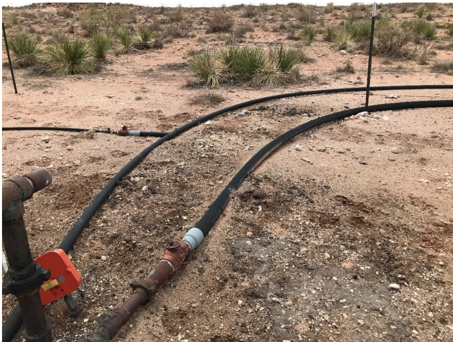
Photo 22: Asphaltine residue observed at the Cato San Andres Unit Well #506 (SW4/SE4, section 02, T08S, R30E).
