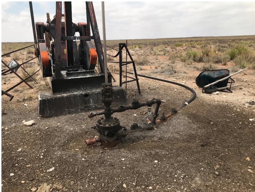
Photo 24: Close up view of the State 32 #005 wellhead, staining present.
