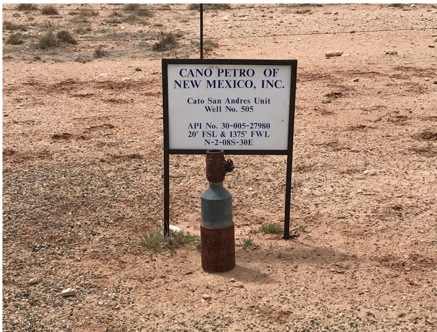
Photo 18: Close up view of well signage and unplugged/open wellbore.
