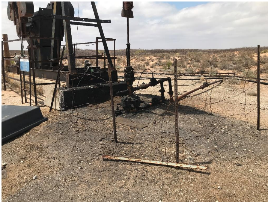
Photo 32: State 32 #002 wellhead, staining present.
