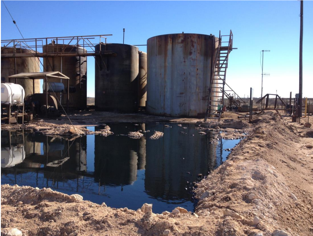
Oil and produced water spill on Sian’s expired business lease located in Lea County.
